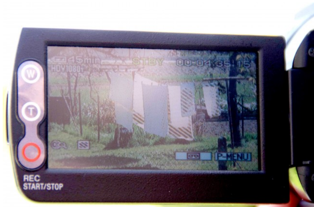
The zebra function marks the brightest spots in the picture
