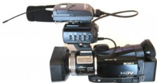
Transmitter, receiver and microphone (left) and receiver attached to the camera
