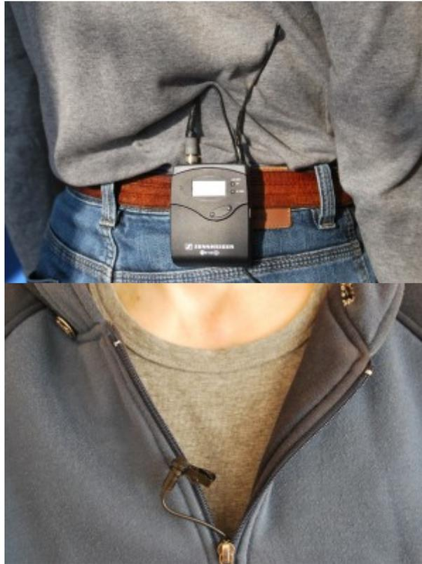
*Transmitter and lapel microphone attached to a person*
